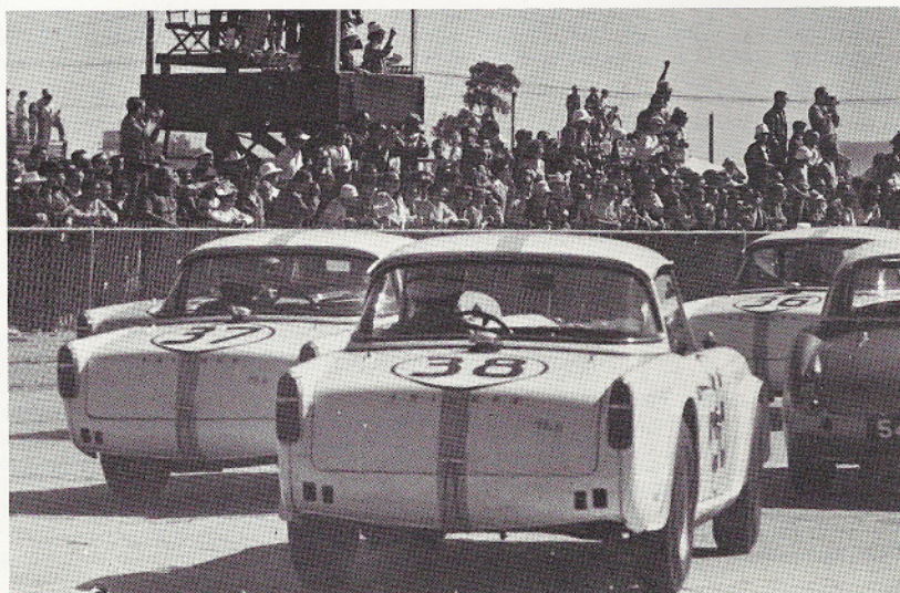
Here can clearly be seen the aluminum strips that were fitted to the front and rear fenders to allow for the wide base wheels, and thus meet F.I.A. regulations.
