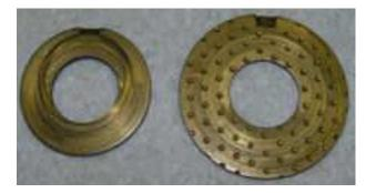
2.00, while it is about 1.57 for the rear one. The thicknesses are approximately 0.068 and 0.107 for front and rear respectively. The current reproduction washers are of inferior quality without the steel backing. The current crop of reproduction rear washers are also about 0.007 thinner than the originals. Reuse your old washers if they are in good condition.
