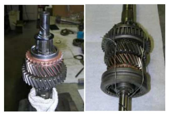
Next, install the synchro rings, both synchro hubs, 1<sup>st</sup> gear with its bushing, and the rear washers. The front synchro hub is installed with the large boss forward and the small boss toward 3<sup>rd</sup> gear. Wire everything together, so it will be ready for installation into the case. The right photo shows the assembly for a three synchro box.
