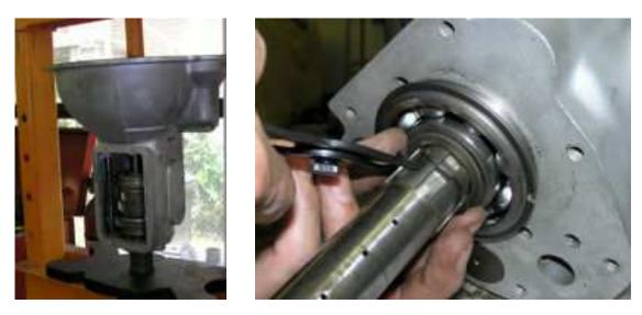
Now install the input shaft assembly and 4<sup>th</sup> gear synchro ring by driving the bearing into the housing. Then turn the transmission top down and work the countershaft gear assembly into position. Make sure the brass washers are in place and slide the countershaft into position. For an early box, this operation will displace the dummy shaft which holds the needle bearings in place. Lock the countershaft and reverse shaft in place. Your transmission should now look like the one below.
