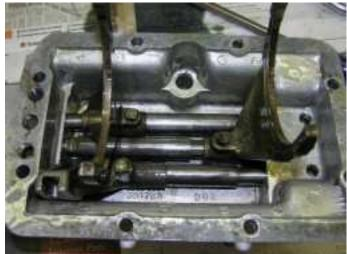
Regardless of these changes the basic mechanical features are similar for all of the top covers. Each of the rails has a detent for each gear and a spring and ball (or plunger) and sometimes a small distance piece or spacer (yellow circles). The detents are to hold the transmission in the selected gear.
