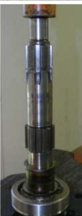
For a four synchro box, you must also check the clearance for the first gear assembly. Install the washer (24), the bushing and the washer (33) on the shaft. Press the center bearing onto the shaft as shown in the photo, then install the washer (35) and the circlip. Once the circlip is positioned, you must turn the shaft around and press the bearing back until it is firmly against the circlip. Now the clearance can be measured with a feeler gauge.
