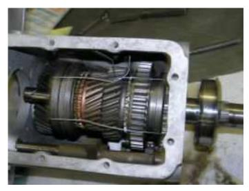
binding. **Don't forget to remove the wire** before pressing the bearing all the way home. Now install the washer (37) and the snap ring. You now must pull or press the bearing back until it is firmly against the washer and snap ring, otherwise the first gear bushing will have no float. The bearing should slide easily into the case.
