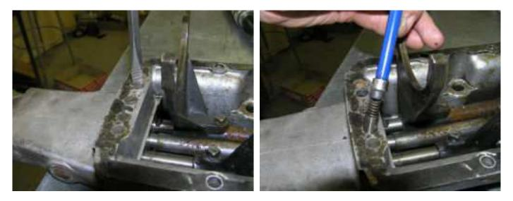
**Adding cover switches:** You will also have to dismantle the cover if you need to add switches. In most models, the switches are tripped by the top of the shift fork when it is beneath the switch, and the switches are easily located by the boss in the top of the cover. To add switches, you will need a 16mm x 2mm metric tap and a 35/64 inch drill. Some of the later TR6 models have
