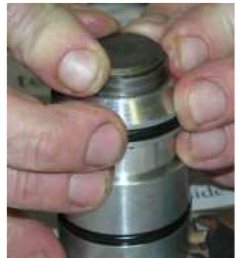
The section on testing describes the use of washers to increase the operating pressure of an overdrive with weak accumulator springs. We normally add one or two 0.060 inch thick washers during the initial assembly as a preemptive measure, since some adjustment will normally be required.
