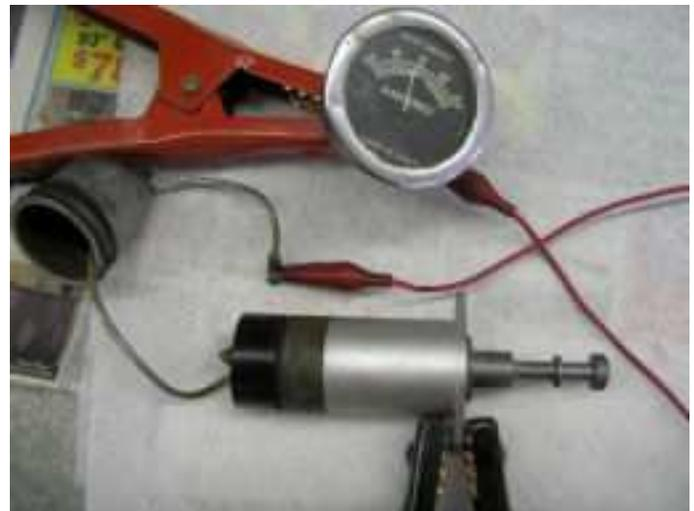
When you apply electricity to the solenoid, you should see a large current briefly and then about 1 amp. When the solenoid does not work, it is usually a problem with one or the other of these circuits.
