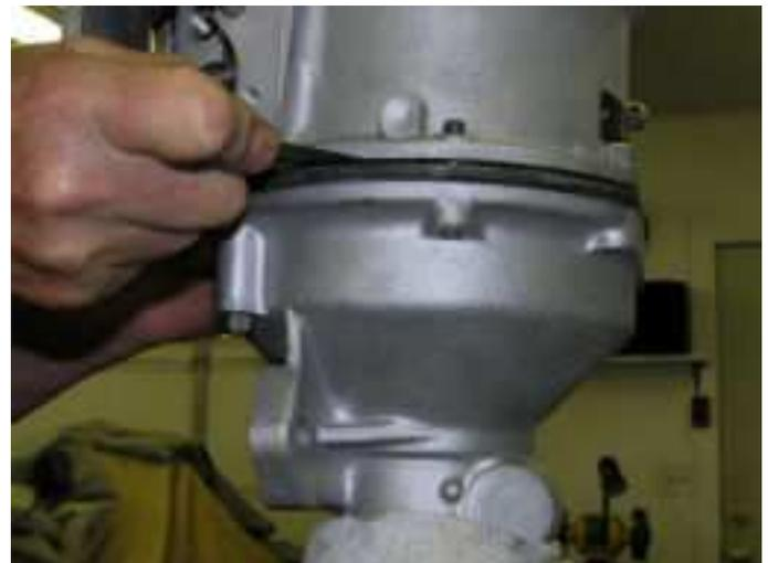
With a feeler gauge the gap was determined to be about 0.070 to 0.072. So, when the 0.091 washer is removed the end float should be about  $0.091 - 0.071 = 0.020$ .
