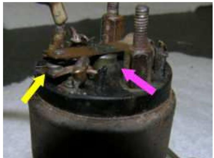
the hold in circuit will not provide enough force to lift the operating lever. Usually, cleaning up the shuttle so it moves freely and/or recontouring the breaker assembly is all that is needed to fix the solenoid.
