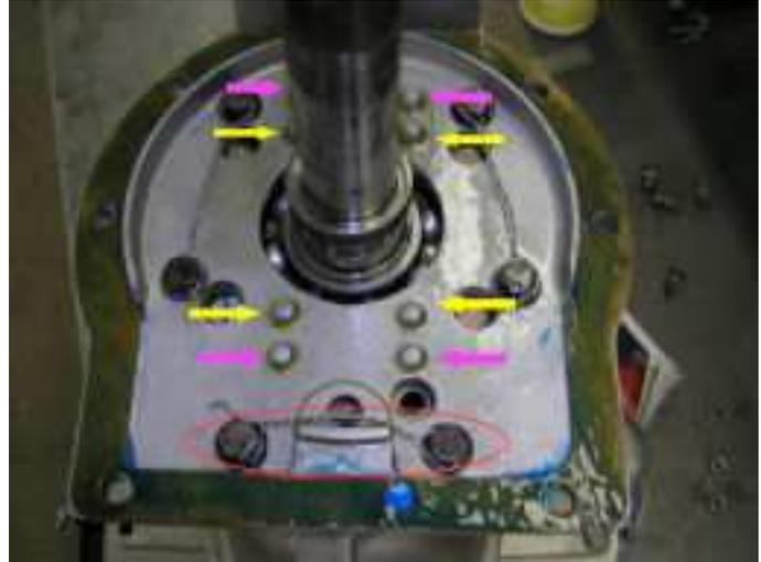
Before mating the overdrive and transmission, we must take steps to insure the pump slides underneath the actuating cam on the main shaft. First, turn the main shaft so the lobe is pointed away from the pump. Use a large C (or G) clamp to compress the pump spring. Then wire it in that position (yellow arrow in photo).
