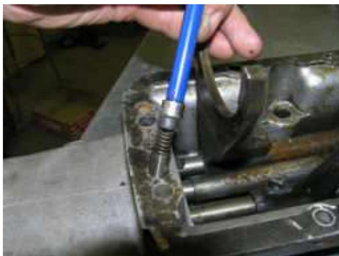
**Adding cover switches:** You will also have to dismantle the cover if you need to add switches. In most models, the switches are tripped by the top of the shift fork when it is beneath the switch, and the switches are easily located by the boss in the top of the cover. To add switches, you will need a 16mm x 2mm metric tap and a 35/64 inch drill. Some of the later TR6 models have
