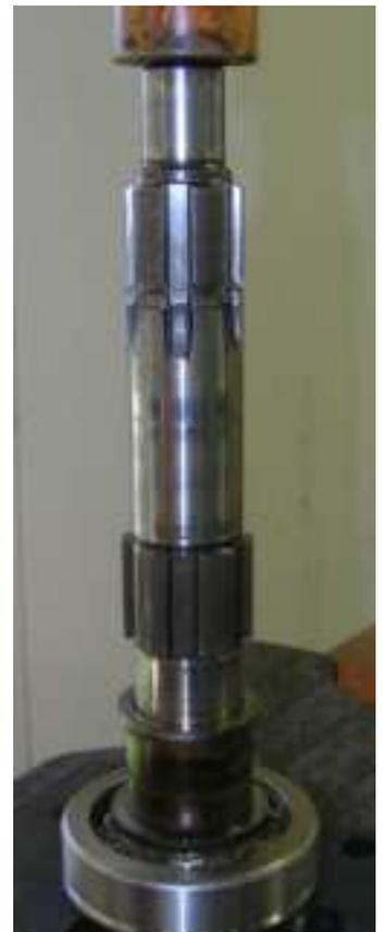
For a four synchro box, you must also check the clearance for the first gear assembly. Install the washer (24), the bushing and the washer (33) on the shaft. Press the center bearing onto the shaft as shown in the photo, then install the washer (35) and the circlip. Once the circlip is positioned, you must turn the shaft around and press the bearing back until it is firmly against the circlip. Now the clearance can be measured with a feeler gauge.
