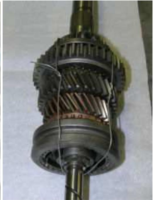
Next, install the synchro rings, both synchro hubs, 1<sup>st</sup> gear with its bushing, and the rear washers. The front synchro hub is installed with the large boss forward and the small boss toward 3<sup>rd</sup> gear. Wire everything together, so it will be ready for installation into the case. The right photo shows the assembly for a three synchro box.
