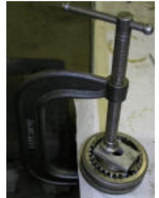
We had not paid much attention to synchro hubs until we worked on a club member's transmission which was popping out of 2<sup>nd</sup> gear. We suspected a broken 2<sup>nd</sup> gear bushing, but that was not the case. In fact, we could see nothing to indicate a problem. Finally, we replaced all the springs in the synchro hubs and top cover. Problem solved.
