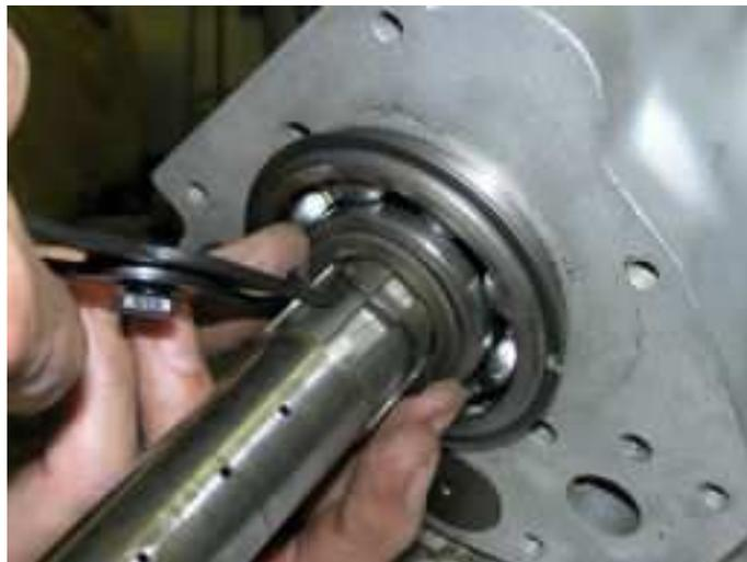
Now install the input shaft assembly and 4<sup>th</sup> gear synchro ring by driving the bearing into the housing. Then turn the transmission top down and work the countershaft gear assembly into position. Make sure the brass washers are in place and slide the countershaft into position. For an early box, this operation will displace the dummy shaft which holds the needle bearings in place. Lock the countershaft and reverse shaft in place. Your transmission should now look like the one below.
